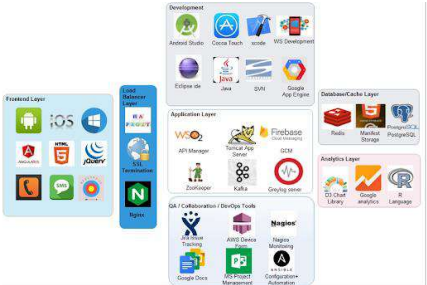
Fig 2 – UMANG Open Source Technology Stack
